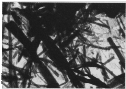
Fig. 4 TEM image of molecular gels for gelator BMDM in diphenyl ether before polymerization, negatively stained by osmic acid ( w = 4.9\% , \times 3600 )
